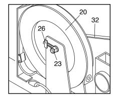
counterclockwise. Make sure that the Flywheel is straight and retighten the M8 Flange Nuts (23). When the Drive Belt is properly adjusted, re-attach the side shields.
